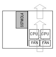
Likely to be Adequate SS7MDL4 board is in line with the airflow created by the main fans as they cool the CPUs. In this scenario, the cooling is likely to be adequate to prevent the occurrence of temperature issues.
